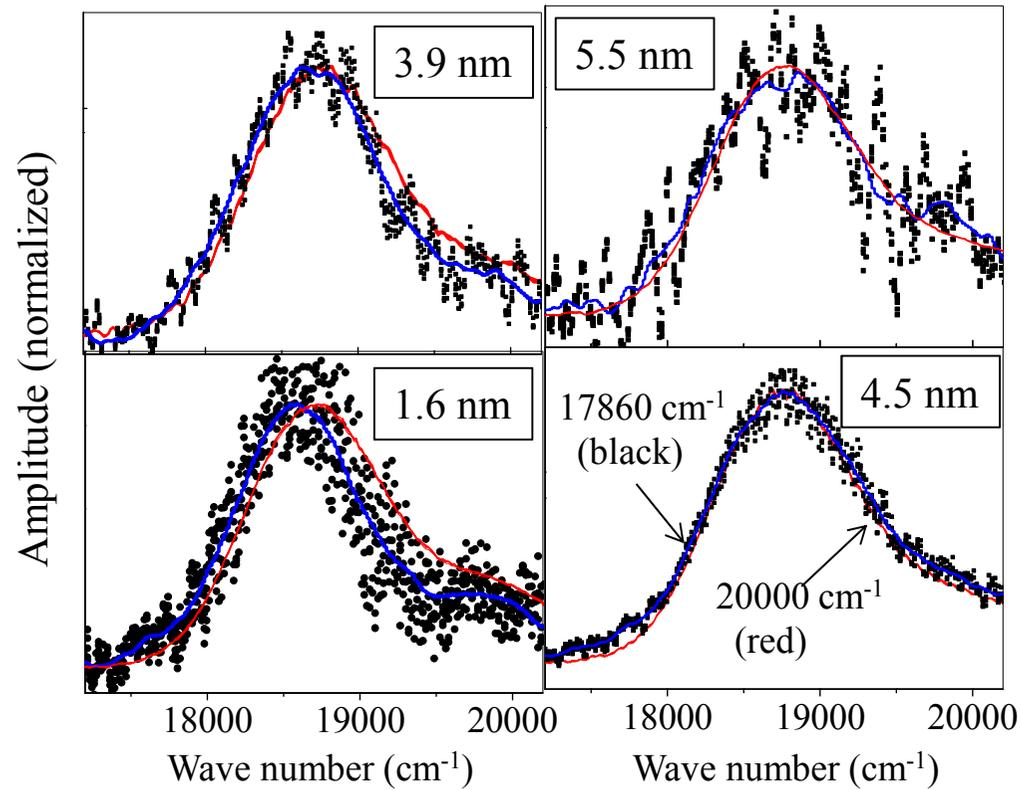
A spectral shift between the two spectra exists at 3.9 nm, whereas the two spectra agree above 4.5 nm.
